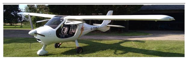
The CT2K is a Three-Axis Microlight – Three-Axis refers to the controls surfaces you would have in a traditional aircraft permitting pitch, roll and yaw. A preconception that people have when they hear the word microlight is the image of a hang-glider with a human and a lawnmower engine suspended under it – this type is called a Flex-Wing. There is nothing wrong with those! But these are also available. Why not give either a go.
